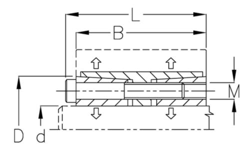
B mm = 155d H8 mm = 520D mm = 615Fit tolerance = Aksel h8, Nav H8 F kN torque = 3900.0L mm = 177M mm = M22P N/mm2 surface pressure on shaft/hub = 146 Surface roughness = R? ?  $3.2 \mu n$ T N m torque = 870000Ts N m bolt tightening torque = 930.0
